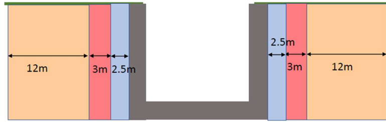
Figure 3: U Section Protection and Exclusion Zones
